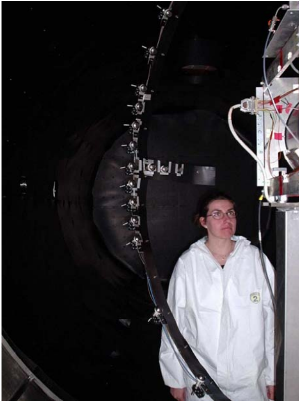
Fig. 7. FPs and RPAs on the diagnostics boom.
